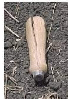
The "control" tool was a wide bladed garden trowel. While the blast did not deform the mild-steel blade, the tool separated and was thrown back a considerable distance (presumably with considerable force). This provides evidence of the need to extend the metal parts of the tool through a handle. The damage to the "hand" holding the tool provides evidence of a need for a hand-guard and some indication of the advantage of using longer tools.
