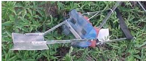
The AVS pick-prod was 7 meters away with its “hand” close by. The tip of the prod was slightly bent but all welds and fixings were undamaged. The hand-guard had been marked by environmental fragmentation but the cover had not been penetrated.
