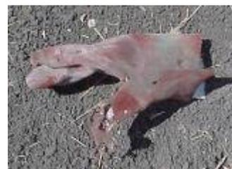
The standard secateurs had separated and the two main parts were found seven meters away and five meters apart. The "hand" holding the short standard secateurs was severely damaged as shown above right.
