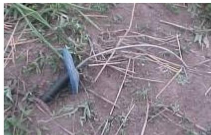
The pick-prod hand had been blown five meters back from the blast and the pick-prod was found about ten metres away. The blade was bent along its length. The fixings and welds of the tool were undamaged. Its hand-guard was marked but no fragments had penetrated the cover of the guard.
