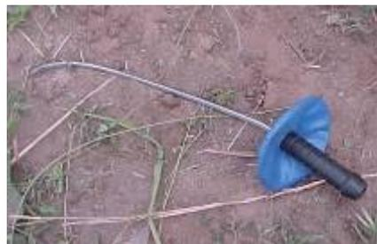
The “hand” holding the second MIT probe was just in front of the crater. The probe itself was seven meters away with a long curve along the length of the blade. The fixings and welds of the tool were undamaged. Its hand-guard was marked but no fragments had penetrated the cover of the guard.
