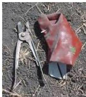
The AVS root-cutter had been blown five meters away and separated from the "hand". The polycarbonate "anvil" of the jaws had been separated and was not found. All the metal parts of the tool were in one piece although the hardened steel cutting blade was deformed. The "hand" holding it had been damaged but not penetrated.
