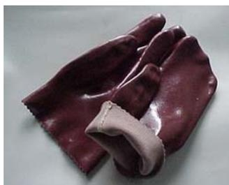
In all these tests the handtools were held in a fabric-reinforced rubber glove with a 0.75mm polycarbonate "hand" inside. The hand slotted into a 5mm polycarbonate "forearm" that was held in position with a stainless steel spike as shown below.
