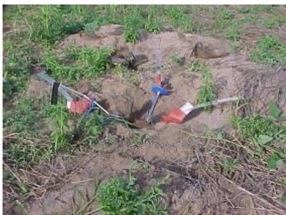
The orientation of the tool was maintained at or below a measured 30° to the ground (the picture on the right includes the protractor).
