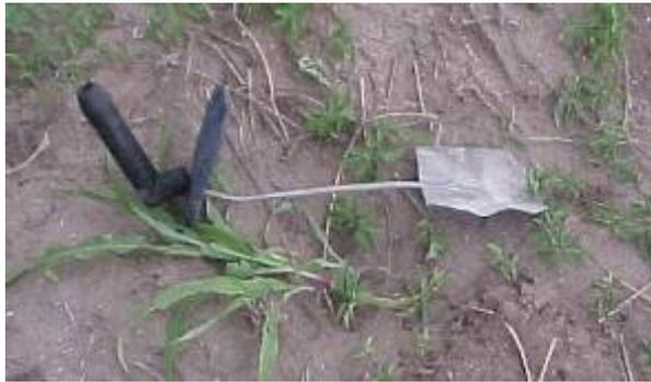
The MIT probe had been blown backwards five meters with its “hand” 4m away to one side of it. The blade had been curved along its length. The fixings and welds of the tool were undamaged. Its hand-guard was marked but no fragments had penetrated the cover of the guard.
