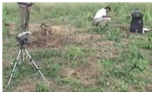
Each tool was placed so that its tip was in contact with the mine. No "interference" between the tools was observed and it is believed that the result would have been substantially the same if each tool had been tested separately.
