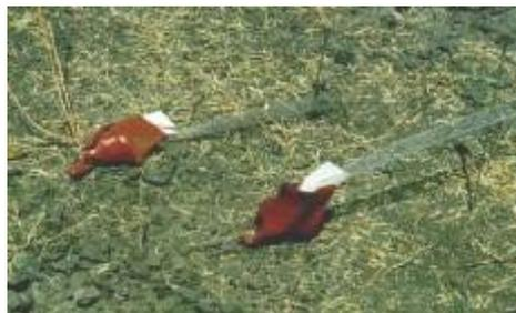
The AVS demining shears remained in one piece after the blast. They had been slightly bent (barely discernible) and still cut undergrowth after the blast. The “hands” holding the shears were undamaged.
